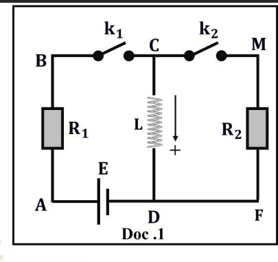
As a result of this process, induced EMF is set up in the coil, such that it opposes the growth of current in the coil. This delays the current to acquire the maximum value.
